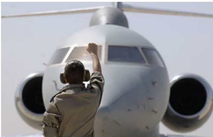
RAF groundcrew in the Gulf brings a Sentinel R1 to a stop as it taxis in from a mission over Afghanistan (Crown Copyright - Cpl Dave Blackburn)
