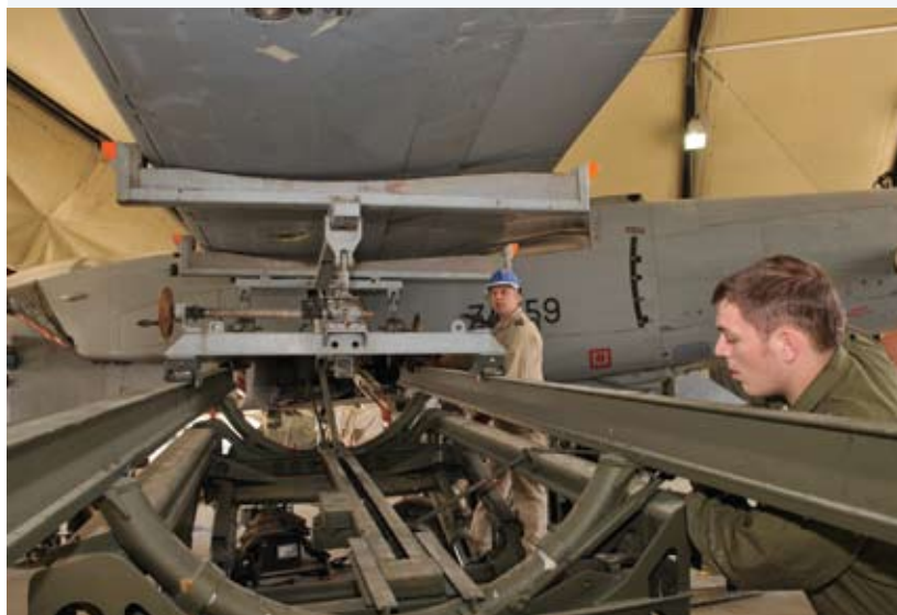
ABOVE - IX(B) Sqn groundcrew remove wings from a Tornado aircraft at Kandahar Airfield so it can be transported back to the UK in a C-17. (Crown Copyright - Cpl Dave Blackburn)
